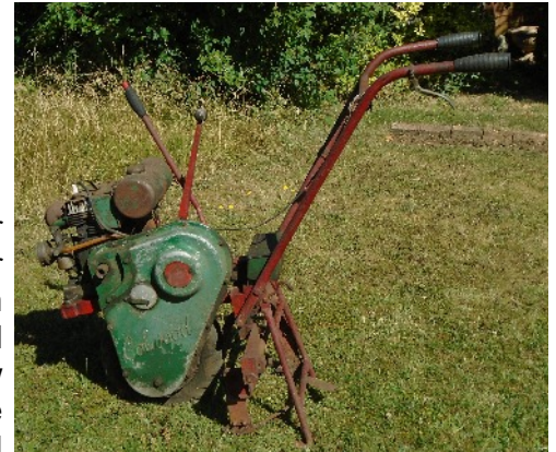
Colwood Motor Hoe, built in the 1940s, single pneumatic wheel, engine turns.
