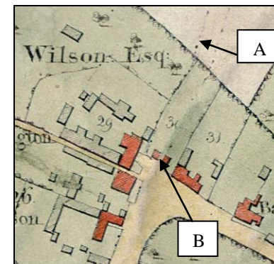
Note the faint outline (A) of the new road to be built. Note also the house (B) which had to be demolished as it was in the way.
